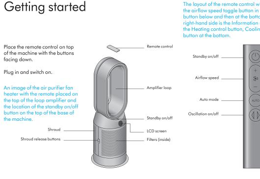
The layout of the remote control with the standby button on the top left, the airflow speed toggle button in the middle left with the Auto mode button below and then at the bottom is the Oscillation button. On the top right-hand side is the Information menu button, then going downwards is the Heating control button, Cooling mode button and then Night mode button at the bottom.
