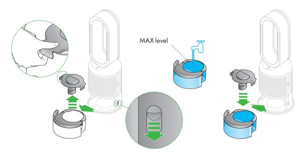
Before you remove the water tank, make sure humidification modes are turned off. Push down the water tank release buttons on the sides of your machine.
