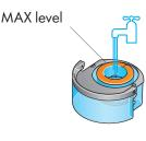
Place the evaporator in the water tank. Fill the water tank to the Max level with cold tap water.
