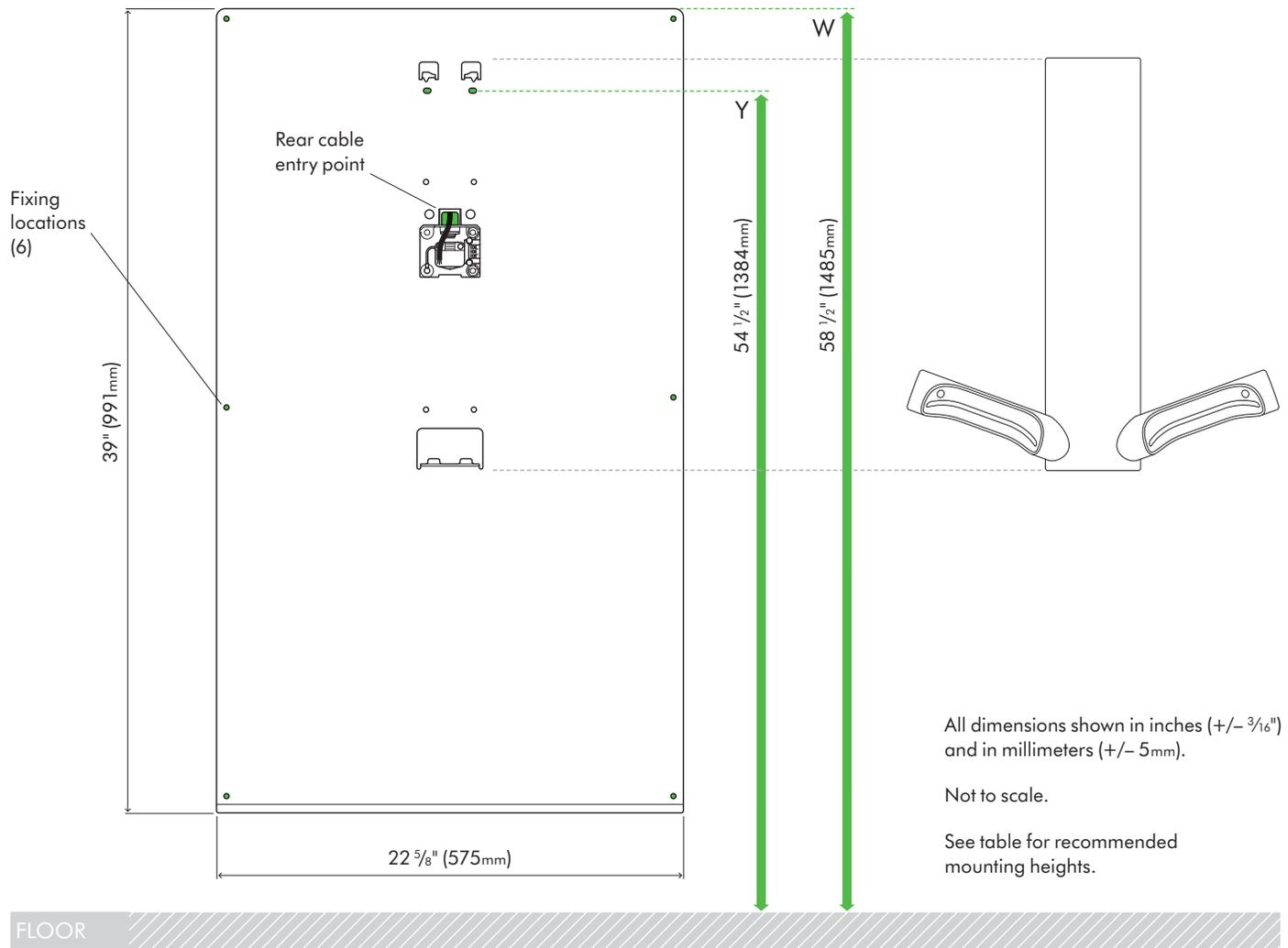
All dimensions shown in inches (+/- 3/16") and in millimeters (+/- 5mm).
