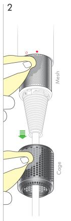
Pull down and away from the machine. Use a lint-free cloth or soft brush to remove any dust or debris from both the filter cage and the filter mesh.
