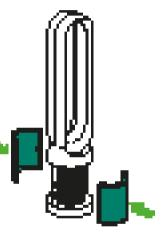
Push the new carbon filters onto the base until secure.
