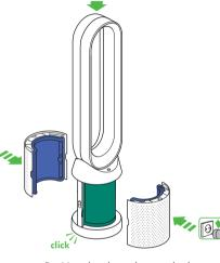
Position the shrouds onto the base and push gently until they click securely into place.
