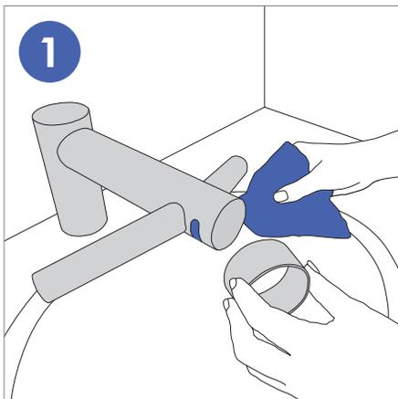
Wipe sensors using soft cloth and non-abrasive cleaner, then place cleaning cap over sensors to prevent air and water from being activated.
