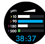
The screen, on the end of the main body, showing a graph of the sizing and counting of the dust particles.
